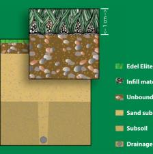
Edel Elite SuperSoft M Infill material: sand 🗱 Unbound/bound base Sand sub base 📰 Subsoil
