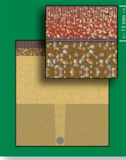
Edel Paddle Pro Infill material: red ceramic sand 📅 Unbound/bound base Sand sub base 📰 Subsoil
